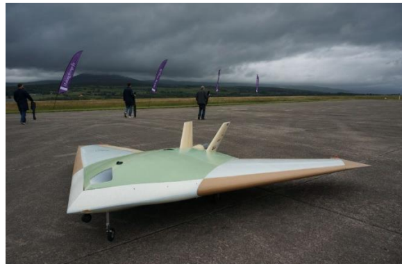
Figure 6: Circulation Control flying demonstrator
