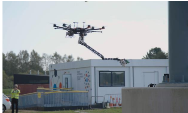
Figure 2: Bridge Inspection UAS
