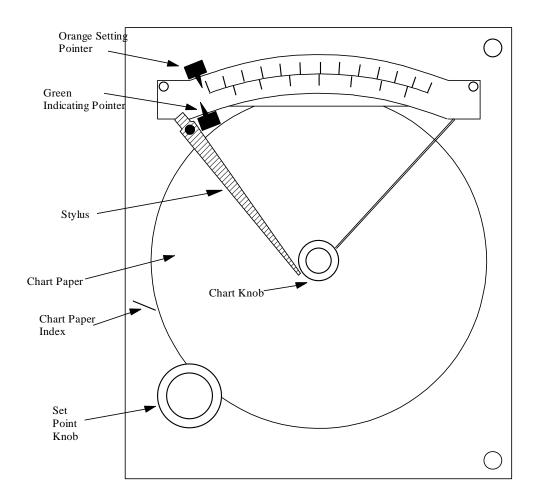
Figure 5.1 Chart Recorder/Controller
