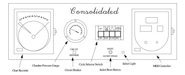
Figure 2.1 The Mark II Controller & Chart Recorder
