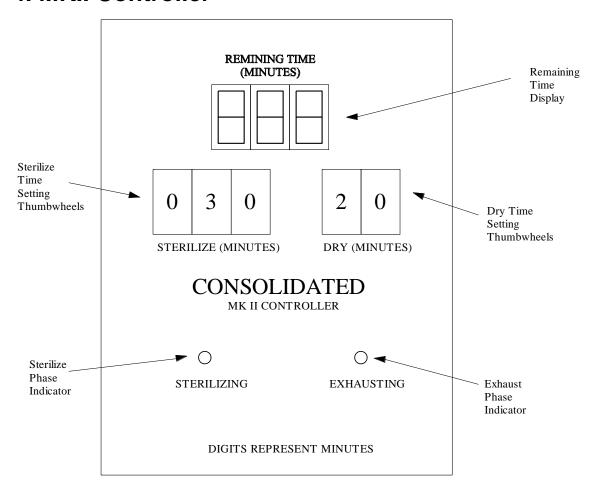
Figure 4.1 MK II Controller Face Plate
