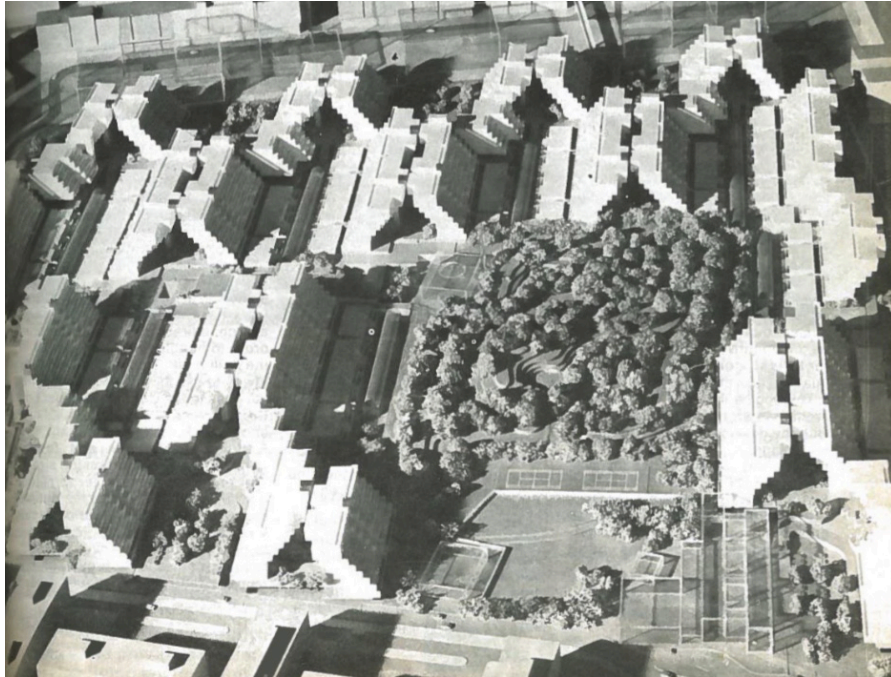
The architect's plan: 900 stacked villas connected by pedestrian 'streets in the air' linking to amenities (Used with permission from the Arthur Erickson Foundation).
